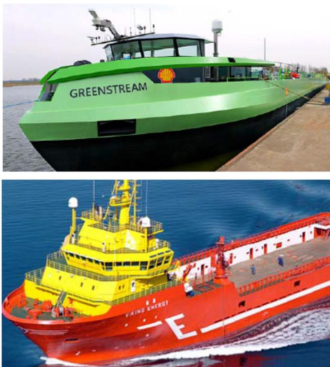
**Fig. 2.** LNG powered: barge on the Rhine (Dutch project 2013) (on the top) and offshore vessel „Viking Energy” (on the bottom) [Rats 2013]
