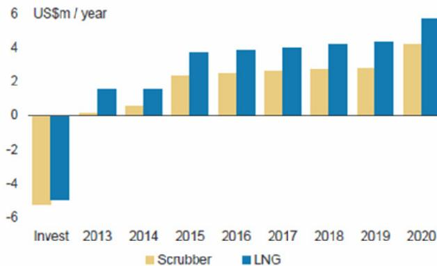
**Fig.1.** Germanischer Lloyd and MAN analysis of switching the engines to LNG [Rats 2013]
