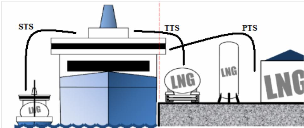
Fig. 3. Possibility of LNG bunkering: STS, TTS, PTS [LNG in Baltic Sea Ports]
